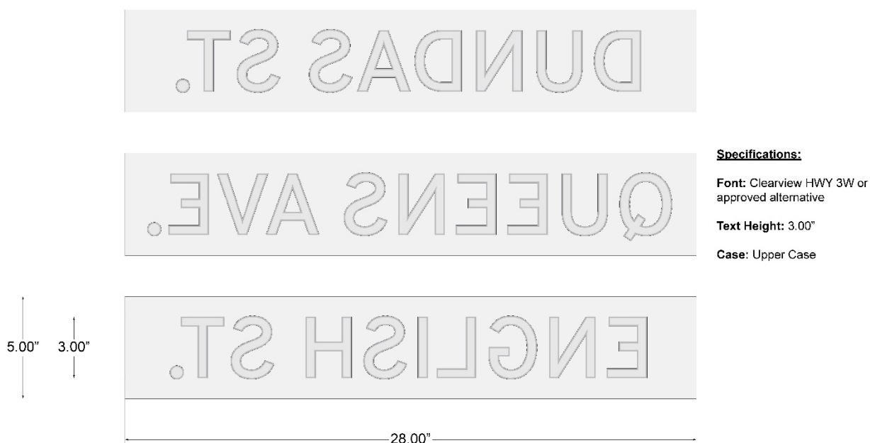
Figure 20.24: Details for Standard Sidewalk Street Name Stamping in Heritage Conservation Districts – Small Width
