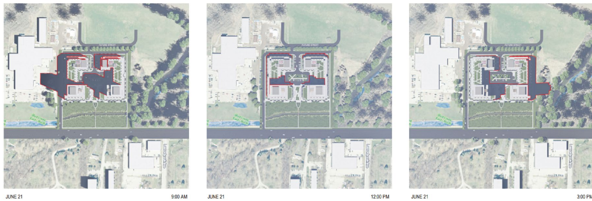
Figure 26 – Shade conditions at the spring/fall equinox (Mar/Sep 21) - 9:00am (L), 12:00pm (C), 5:00pm (R)
