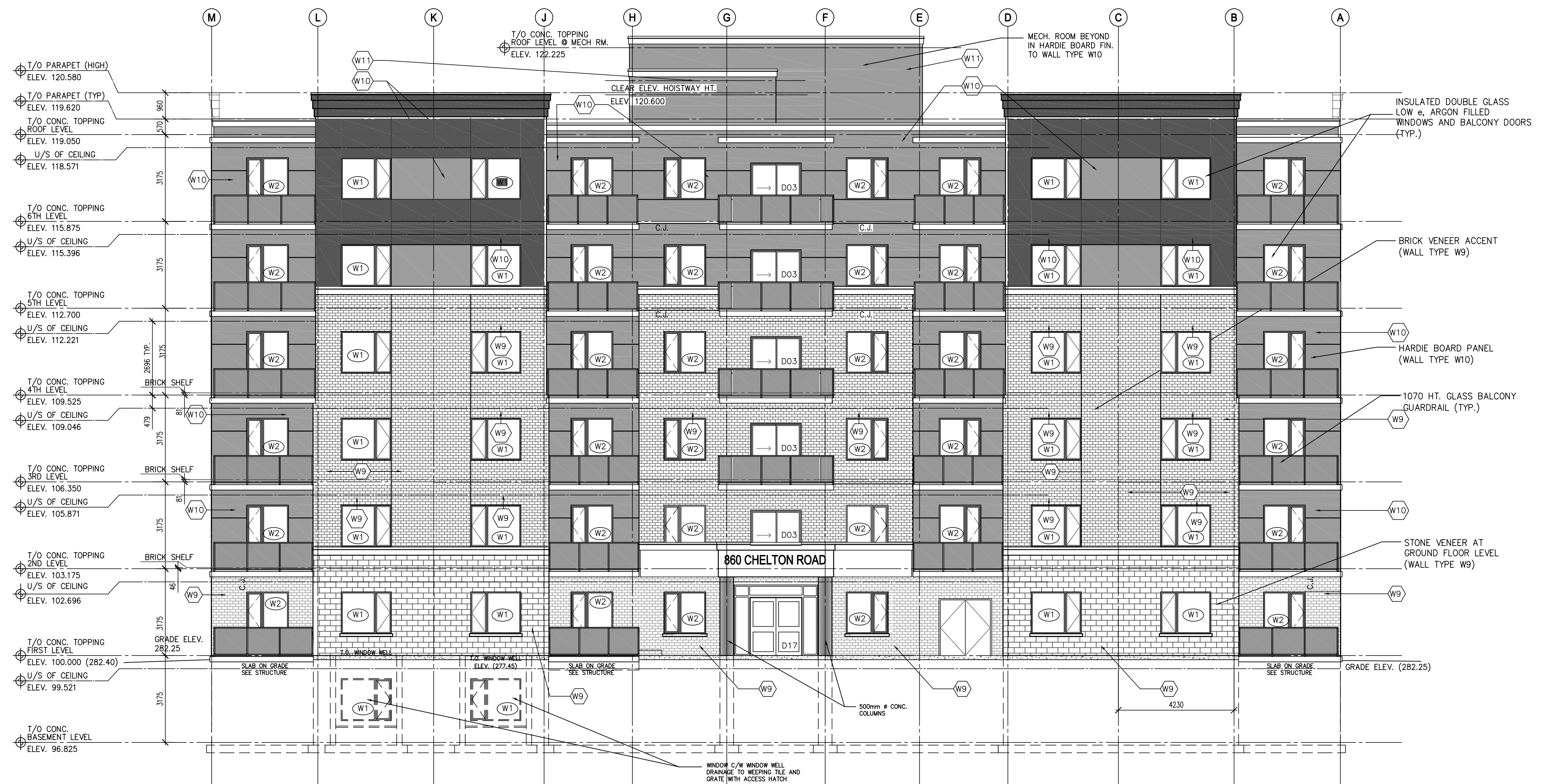
SOUTH ELEVATION - BUILDING A SCALE: 1:100
