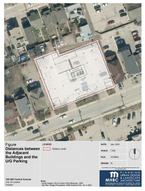
Figure 32: Overlay of parking garage on subject lands and approximate distance between the limits of the parking garage and the existing adjacent buildings and structures (Source: MHBC, 2023).
