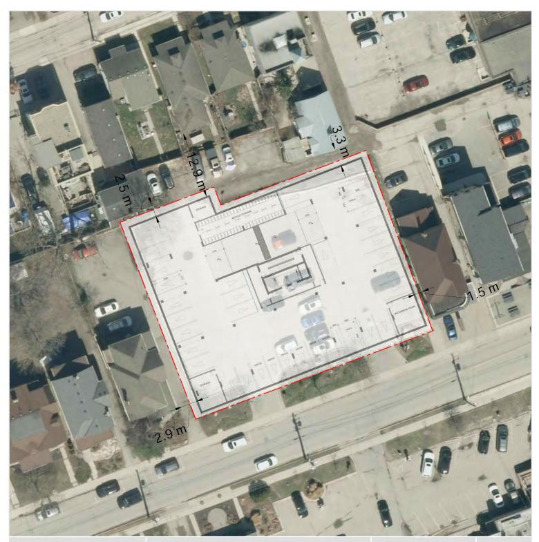
**Figure** Distances between the Adjacent Buildings and the U/G Parking
