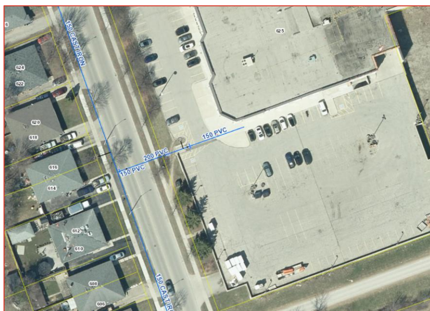
Figure 1 Existing water main along Mornington Ave at the subject site
