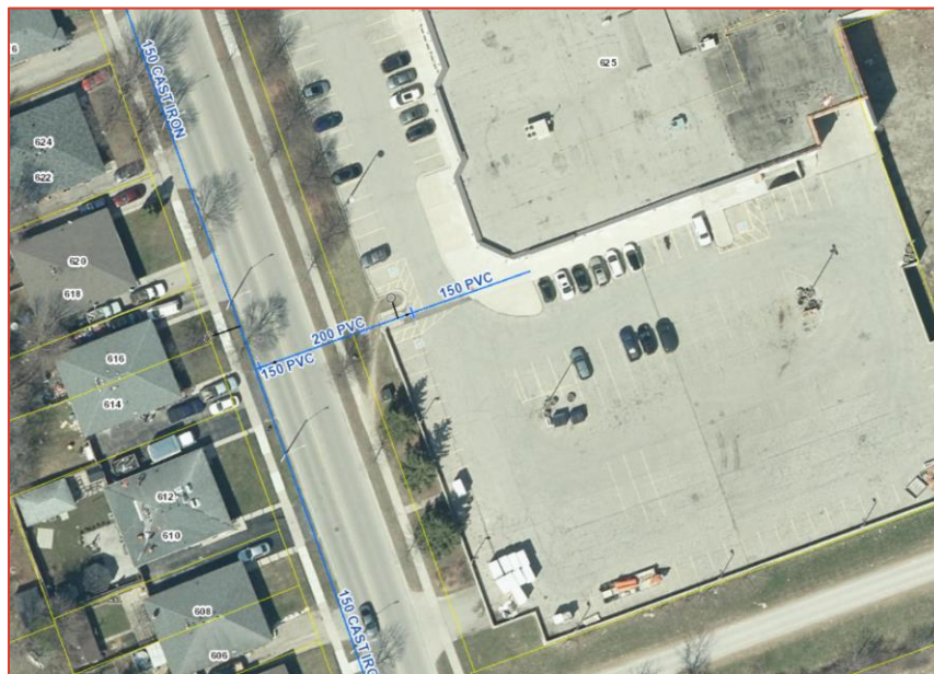
Figure 1 Existing water main along Mornington Ave at the subject site
