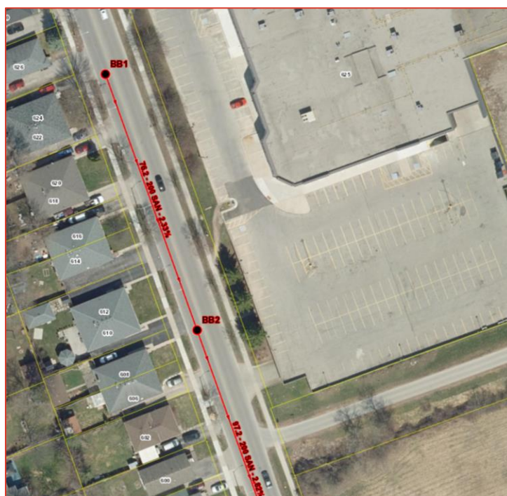
Figure 1 Existing sanitary sewer along Mornington Ave at the subject site
