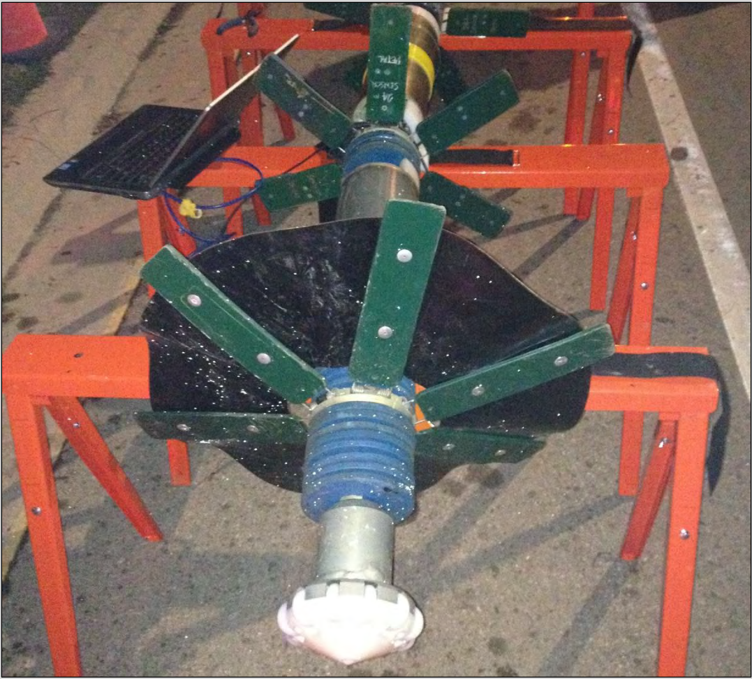
Pipe Diver used to inspect live watermains
