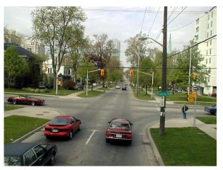
Overhead electricity and communications cables provide easier access but are vulnerable to tree/ ice damage and detract from the streetscape's experience.
