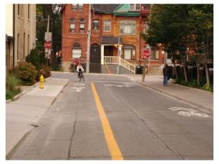
A **contraflow bike lane** accommodates two-way bicycle operation on a one-way street in Toronto.
