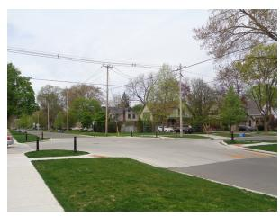
A **raised intersection** in London helps to reduce travel speed through the intersection.
