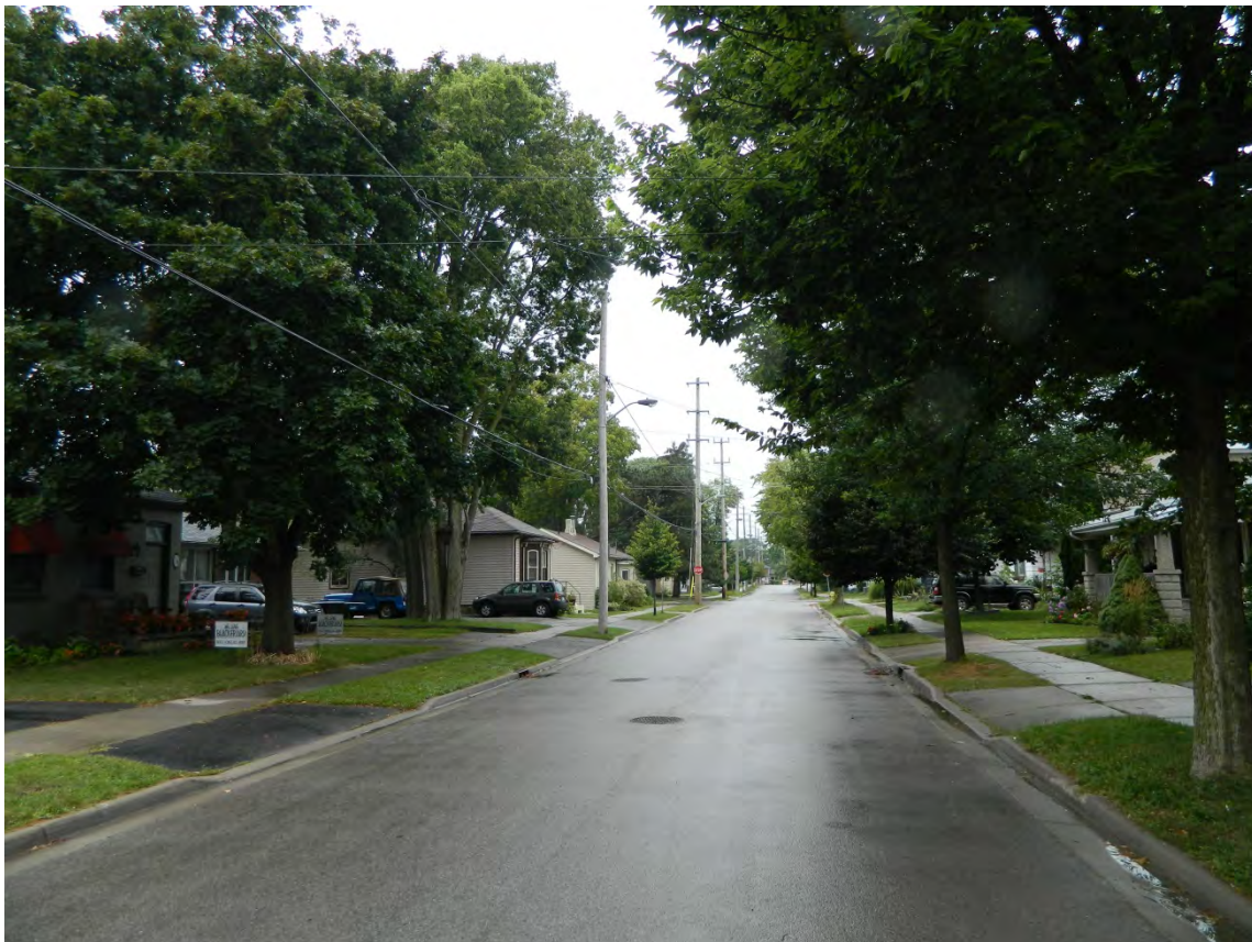
Figure 18: Typical residential street cross section: narrow, two-lane road; grassed boulevard (with or without street trees); and sidewalk.
