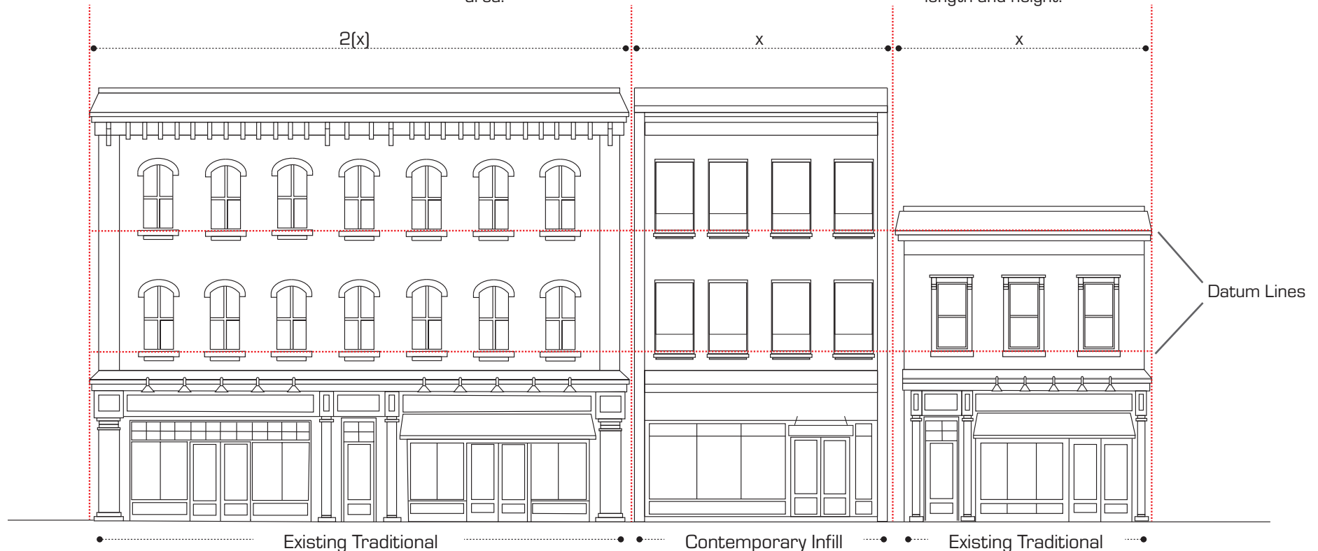
Diagram detailing how infill development can seek to match and maintain the existing rhythm set out by existing buildings.
