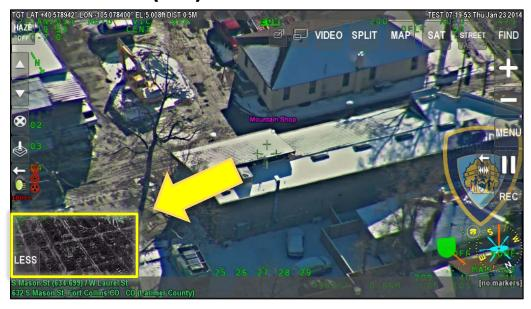
ARS can display two video inputs on-screen simultaneously in a Picture in Picture (PIP) format. In the example above, the PIP window is displayed in the lower left corner. The PIP window location can be selected from the menu. PIP selection buttons are located along the top center of the screen and allow the video inputs to be swapped and the PIP window to be turned on and off. The first two video inputs connected to ARS can be displayed though the PIP feature.
