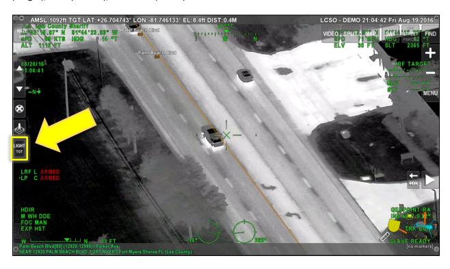
Searchlight position, whether being commanded by ARS or not, is indicated via the icons in the lower right corner of the ARS screen. The searchlight's elevation and azimuth will show as a white cone superimposed on the camera elevation and azimuth orange cone. In the example below, the searchlight is operating in TGT mode where the camera and searchlight position are the same.
