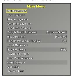
The ARS menu is accessed by pressing the MENU button or by using the M key. Use the menu to select features and layers, to configure the system, or to format items shown on-screen. Menu items in white text are selected for display and items in black text will be hidden from view. While the menu is open, information about the selected menu option will display in the lower right corner of the screen. Press the back button (upper left) or use the **Backspace key** to return to the previous menu.
