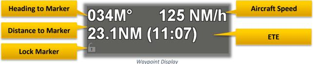
Select On w/Arrow to show the waypoint display with an on-screen arrow/overhead compass showing direction to the active marker as well as the azimuth where the camera is pointed.
