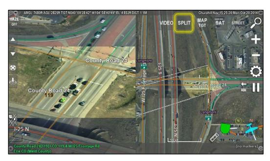
Split mode allows the operator to simultaneously view both the live video feed as well as the map layer. It is enabled by pressing the **split button** on the screen or by pressing the **F5 key**.
